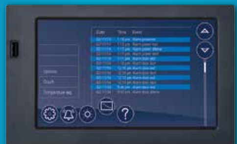
Event and data logging with easy downloading via convenient USB port
